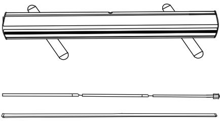
A diagram showing the parts included in the kit: one banner bar with feet attached, one long banner, and two feet.
